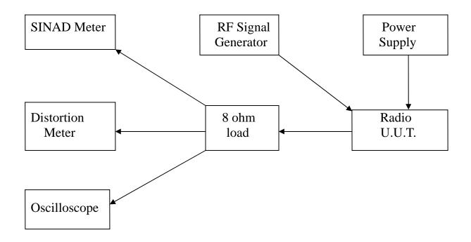
**Note:** U.U.T. = device under test
